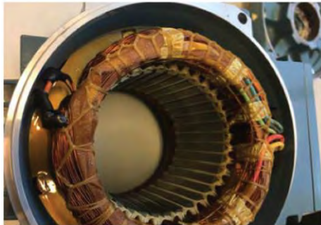
(b) stator-turn fault
