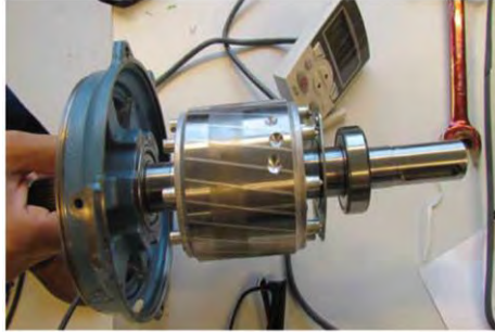
(a) broken rotor bars
