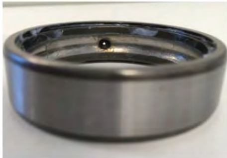
(c) bearing outer race fault
